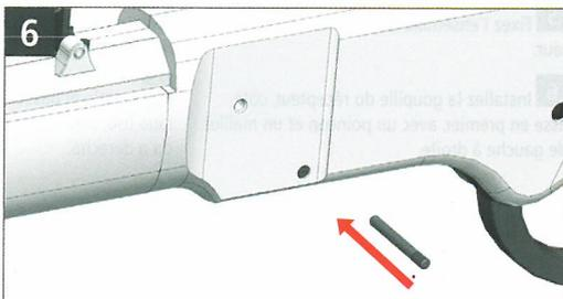
Install the receiver pin, smooth side first, with a punch and mallet from left to right.\*
