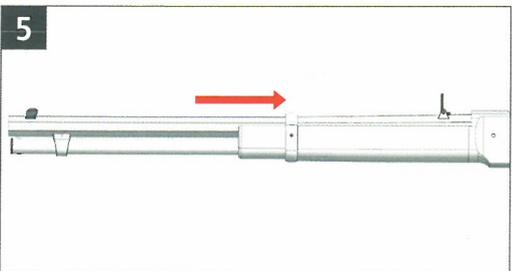
Attach the front barrel assembly to the receiver.\*
