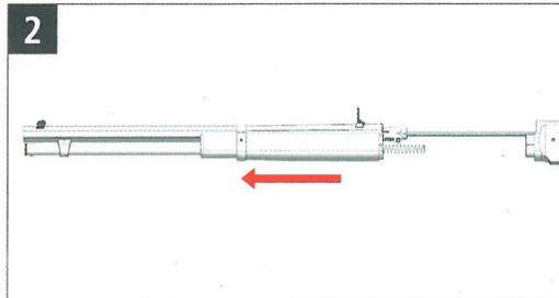
Slide the entire front barrel assembly off to separate it from the receiver.\*
