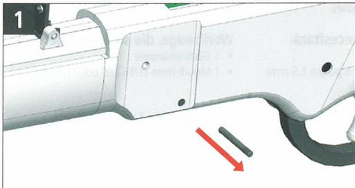
Remove the receiver pin with a punch and mallet from right to left. Take care not to damage the surface of the receiver. Receiver damage is not covered by warranty.\*
