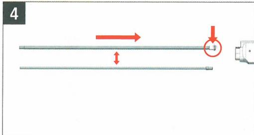
Attach the caliber adapter to the inner barrel you are preparing to install. Insert the inner barrel with installed caliber adapter into the front barrel assembly.\*
