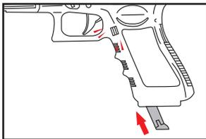
Reinsert the magazine into the Airsoft gun, pushing it into the Airsoft gun until a click is heard.
