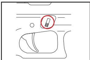
Push the Safety to the "Off Safe" position. The Airsoft gun is now ready to fire. Pull the trigger to shoot with the Airsoft gun. After firing, return the safety to the "On Safe" position.
