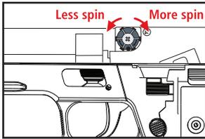
Unmount the top of the gun. Press and hold the release button and take the top off. Gradually turn the lever from left to right and fire a round or two to see the effect. Continue to adjust until the BBs fly straight/horizontally. Perfect Hop-up is applied when the BBs fly straight.
