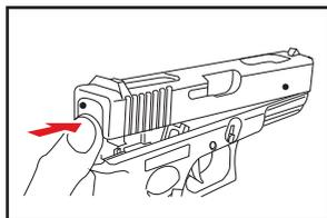
Unmount the top of the gun. Press and hold the release button and take the top off.
