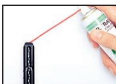
Add a few drops of silicone oil on the BB located in the BB loading hole. Reinsert the magazine into the Airgun.
