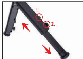
The length of the legs can be adjusted by pulling them out. The bipod has 6 positions. (1) To close the legs, press the leg release button. (2) The leg length can be locked in position by turning the lock screw clockwise.
