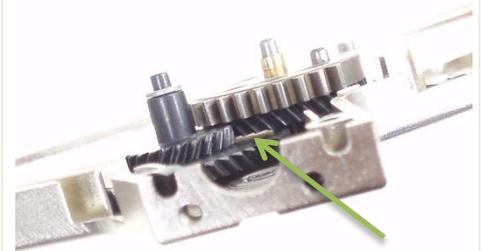
8. Filling the gap between spur gear and right side of gearbox
