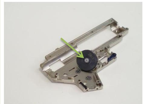
4. Filling the gap between spur gear and right side of gearbox
